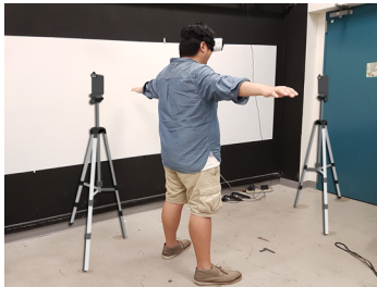
Figure 2: The hardware setting of our system. It includes one mobile head-mounted display and two smartphones attached on tripod.
