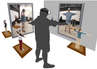
Figure 1: Scenario of this guiding system. (a) Mobile HMD with monocular video see-through (b) Surrounding virtual instructor (c) Augmented mirror which could provide visual feedback such as reflective materials (d) rear camera of smartphone
